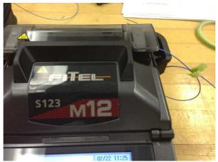
Figure 2 - Close the lid and splice the fibers.
