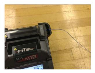
Figure 4 – Place the splice and heat shrink sleeve in the heater.
