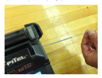
Figure 3 – Slide the heat shrink over the splice.
